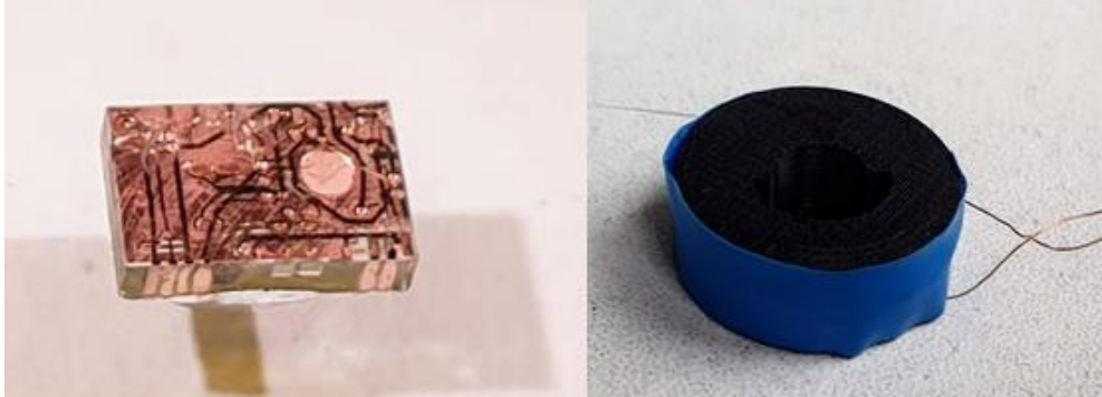
Power module with LTC3106 buck-bust converter (8.1 x 5.2 x 1.5 mm 3 ) and coil
